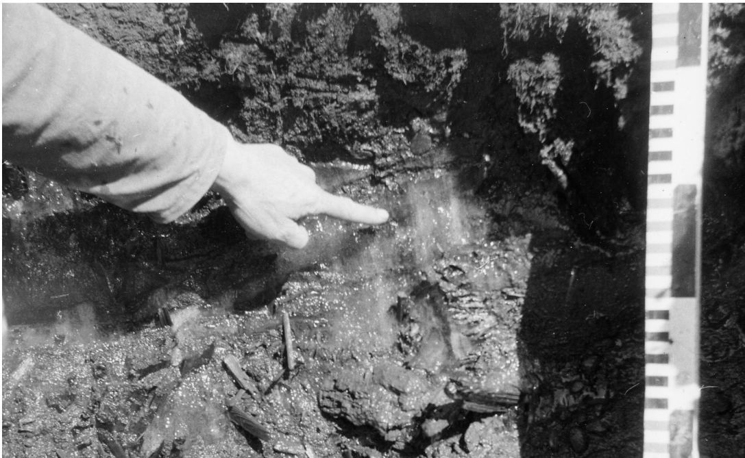
Figure 20. Profile B, B5 picket, blown up. The ice interbed 10 to 15 cm thick is easily visible. View from the west.
