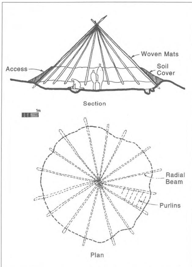
Figure 4. Structural Strategies Type: D Radial Beams
