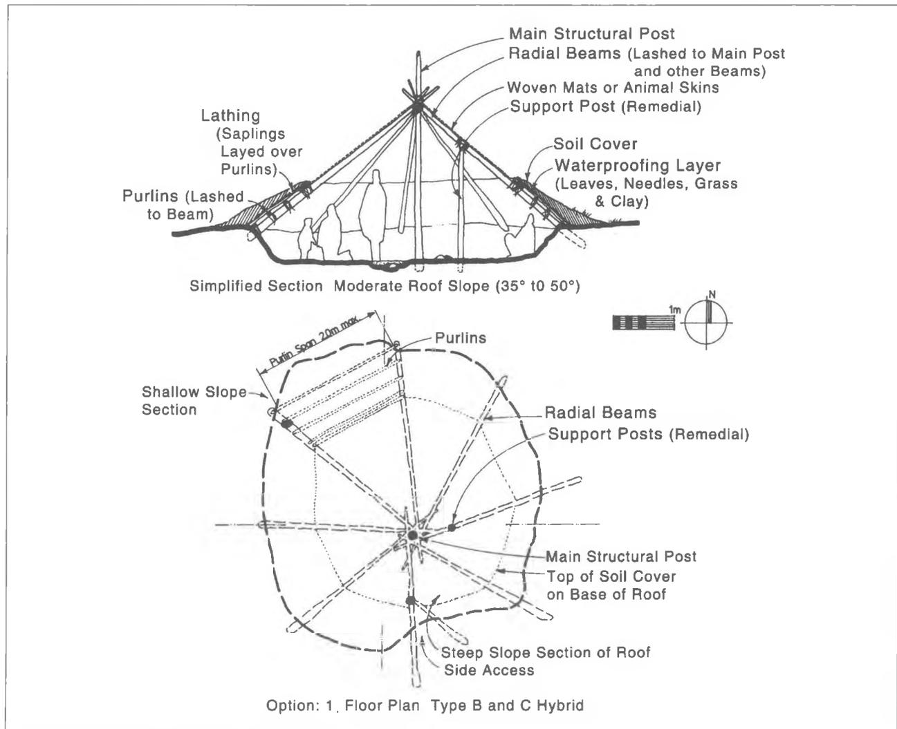
Figure 15. Selected Layout HP 9 Floor Plan and Section
