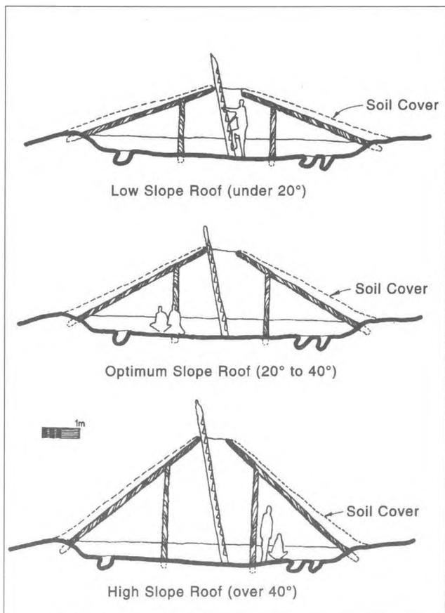
Figure 5. Slope Comparisons Types A and B
