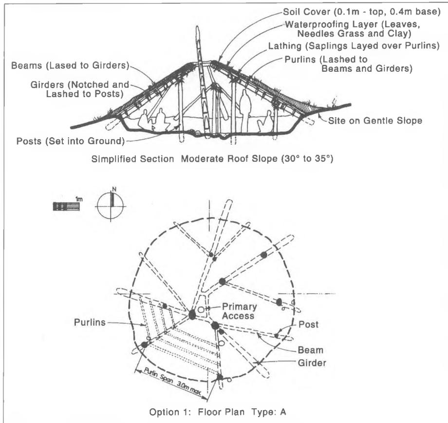
Figure 16. Selected Layout HP 12 Floor Plan and Section
