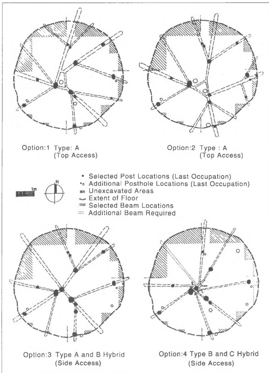
Figure 11. Structural Options HP 12 Floor Plan
