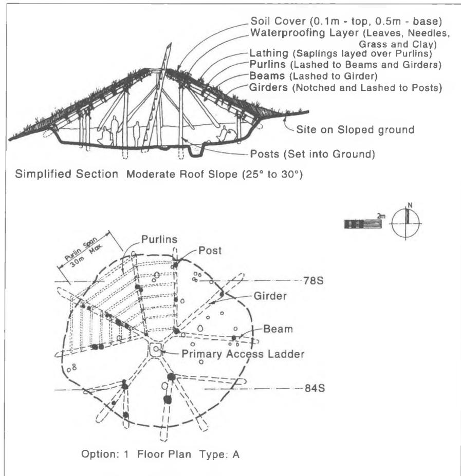
Figure 13. Selected Layout HP 3 Floor Plan and Section
