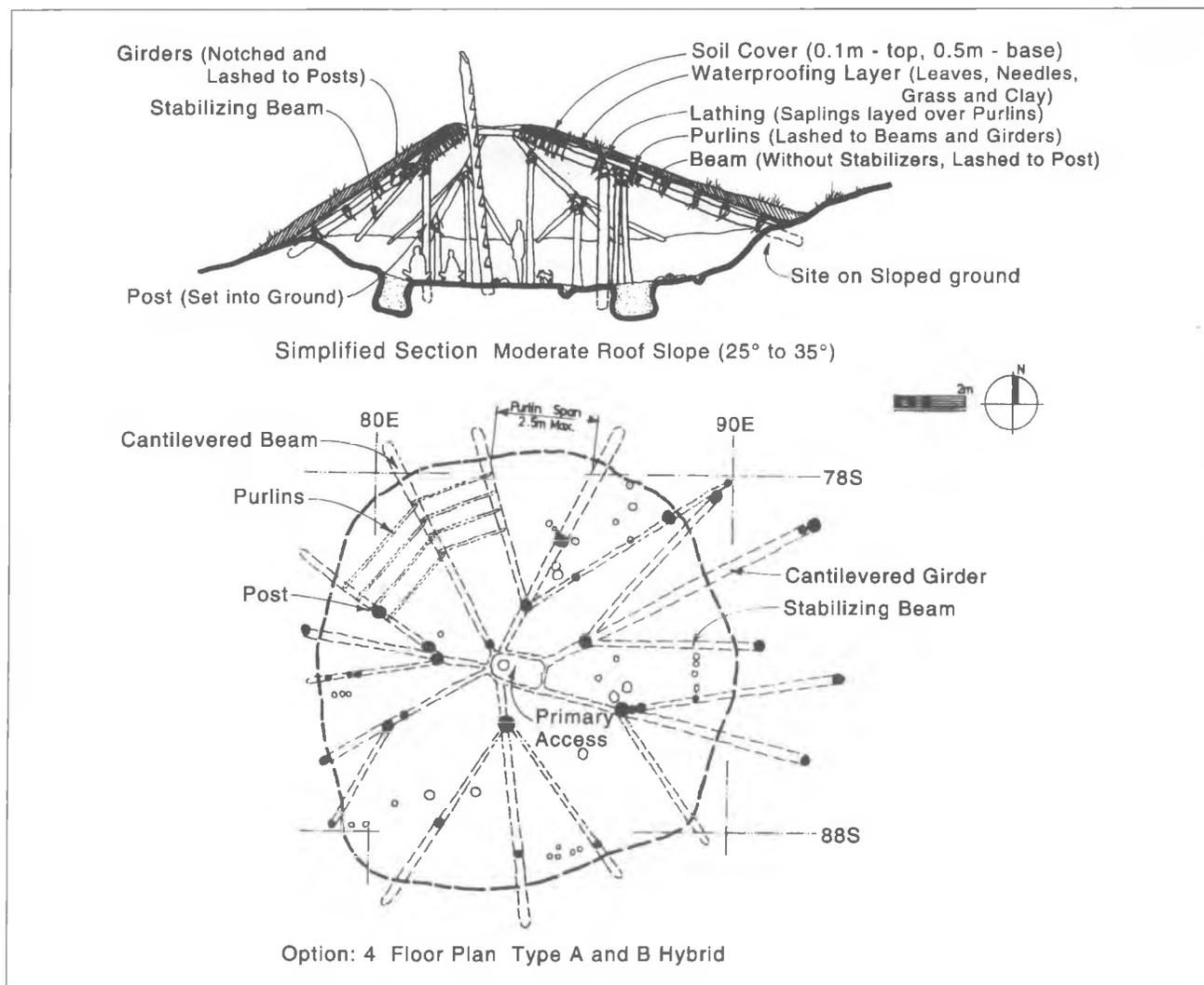
Figure 14. Selected Layout HP 7 Floor Plan and Section
