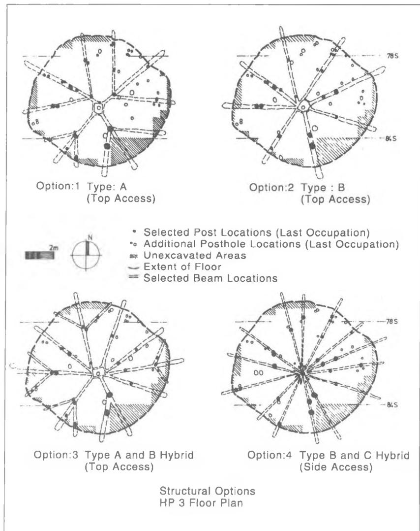
Figure 8. Structural Options HP 3 Floor Plan
