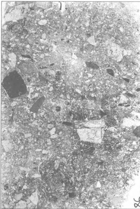
Figure 9. Sample KC-86-26a. This sample reveals loosely packed rock fragments at the top, overlying a similar layer but which is richer in charcoal, which in turn overlies a slightly finer grained, denser material; the latter representing cicada burrows. PPL; length of sample = ca. 8.5 cm.
