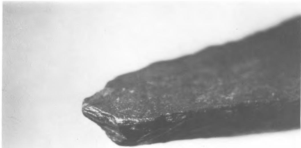
**Figure 21.** Pronounced rounding and moderately bright polish on the distal tip of prehistoric specimen "Y-1". Magnified 8 X.
