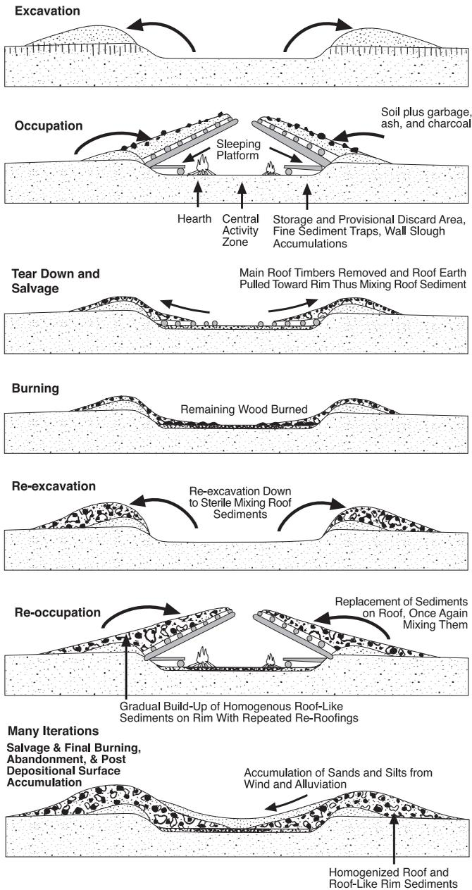
*In each re-roofing cycle of earth-covered houses, refuse accumulated on the roof and on the rim during occupation. All this material was then piled on the rims while the old roof was being replaced, and much of the soil and refuse from the previous occupations was then thrown on top of the new roof or left churned up on the rims. In this way, increasing amounts mixed together and accumulated over time in the roof deposits and in the portion of the rim affected by re-roofing activities.*
