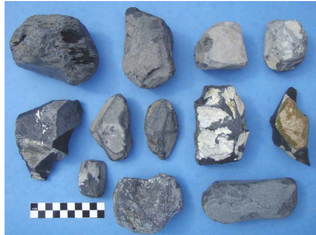
Figure 3-7. Cobbles and pebbles of Maiden Creek dacite showing range of clast forms and typical cortical surfaces.
