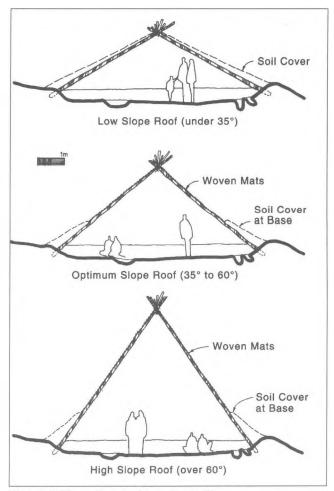
Figure 7. Slope Comparisons Type: D
