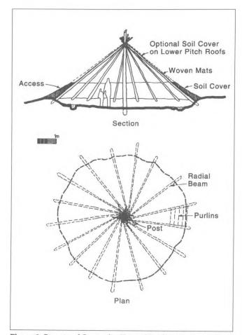
Figure 3. Structural Strategies Type: C Radial Beams and Post
