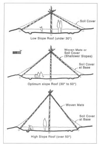
Figure 6. Slope Comparisons Type: C
